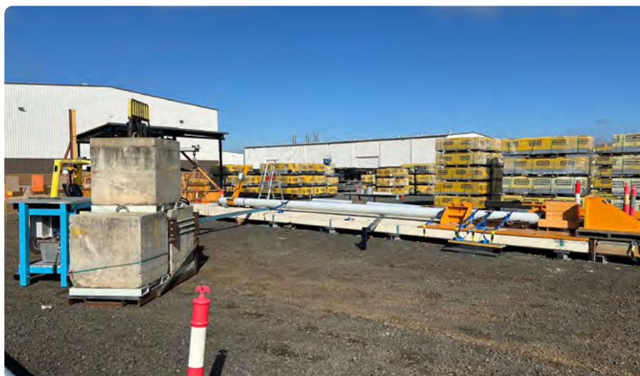
Figure 23 – Combined load test on the Wagners CFT utility pole
