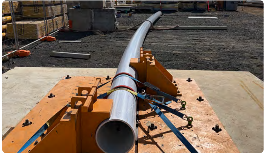
Figure 5 – Testing of the cantilever full-scale flexural test
