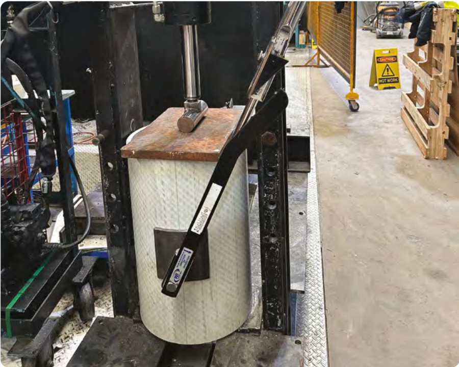
Figure 9 – Bolt torque test setup
