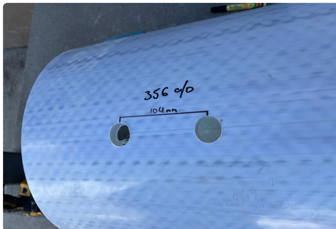
Figure 3 - Pole specimen with bolt holes spaced at 4d_{\text{hole}}
