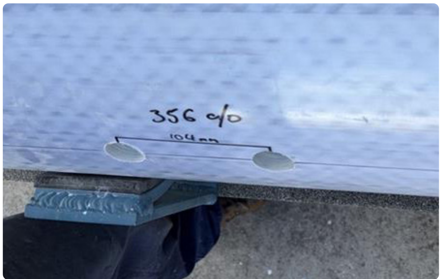
Figure 4 - Drilling for rotational angle and hole distance
