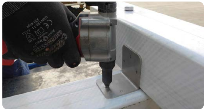
Installing rivet using rivet gun
