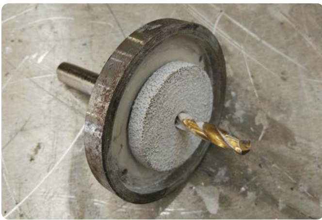
Countersinking tool for decking fixing
