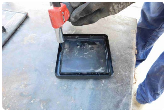
Running butane burner around the edge of endcap
