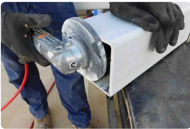
Grooving the internal perimeter of composite member
