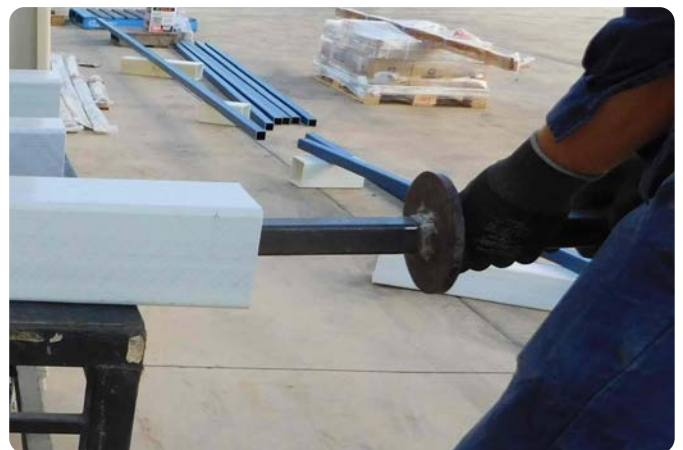
Pushing insert using manual push bar
