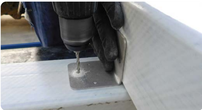
Drilling of hole before riveting
