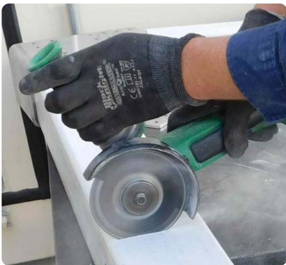
Cutting of FRP material using angle grinder with diamond coated blade
